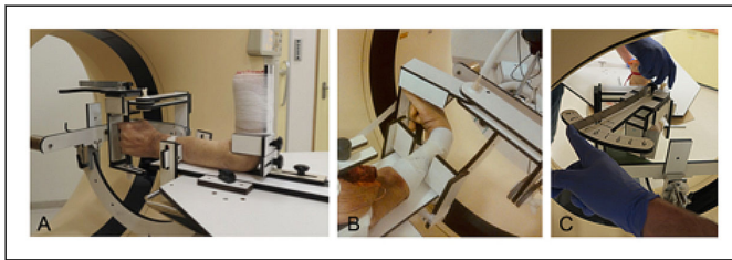
Figure 3: Frame set-up with an example cadaveric arm. Neutral position (A), Flexion (B) and application of 1 Nm of static force (C)
