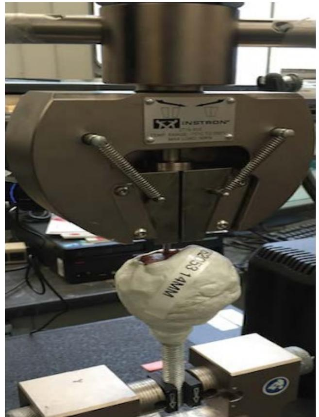
**Figure 4:** Testing apparatus for screw pullout of cadaveric specimen.
