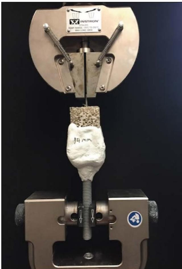
**Figure 3:** Testing apparatus for screw pullout of synthetic bone composite.
