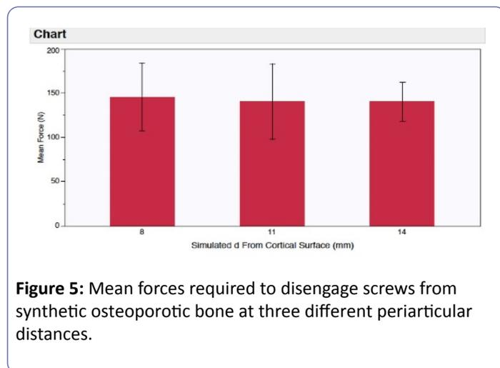
**Figure 5:** Mean forces required to disengage screws from synthetic osteoporotic bone at three different periarticular distances.
