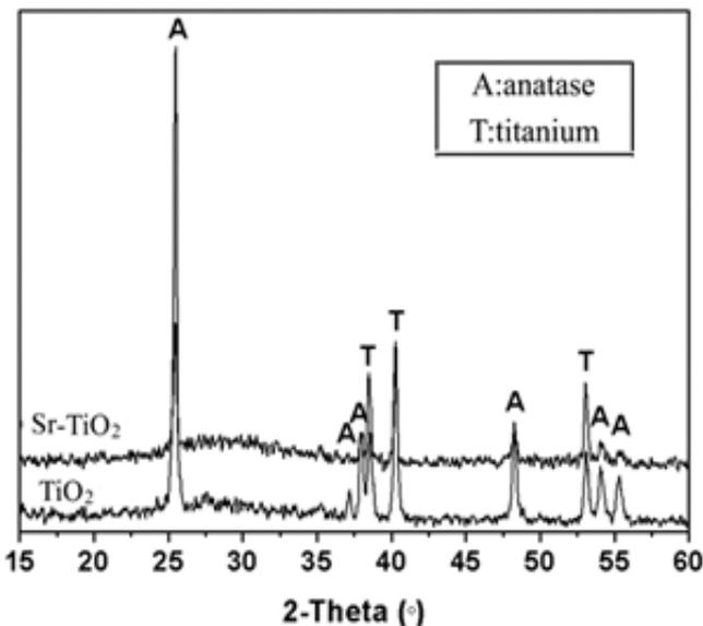
**Figure 3** XRD patterns of  $\text{TiO}_2$  and  $\text{Sr-TiO}_2$  coatings.
